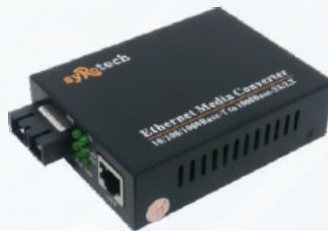
GOMC-8512-02 10/100/1000M MM Dual Fiber, 850nm, SC, 2Km
